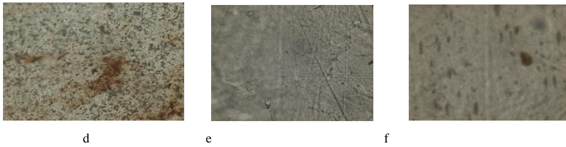
Fig 6 Optical micrograph (magnification 40x) after 0hr irradiation a) PP Fd 0.2 W% b) PE Fe 0.2W% c) EPU Fe 0.2W% d) EPR Fe 0.2W% e) PP Is 0.2W% f) PE Is 0.2W%
